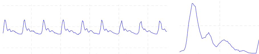
Figure 47 Under damped arterial waveform, detailing enlarged section of trace, achieved by using 2m long tubing. Note the extenuation and additional features as a result of the added harmonics.
